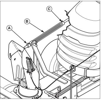
Figure 7. Adjusting Lift Rod
